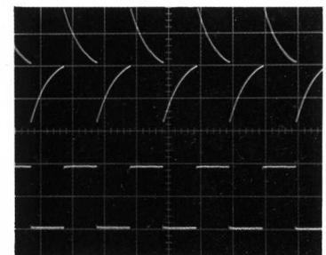
A 10Hz square wave oscilloscope comparison of AC (top) and DC (below) amplifier output signals. The DC amplifier shows no waveform deformation.
