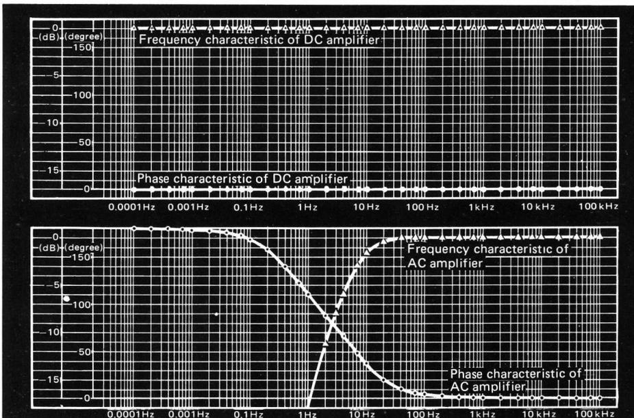
Only a DC amplifier's frequency response is completely flat from 0Hz to 100kHz.
