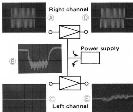
The disadvantage of a single power supply. A) A transient input signal is applied to the right channel. B) This signal affects the normally stable power voltage. C) The left channel has no input signal. D) The original input signal is amplified. E) When the same power supply (B) is used for both channels, a spurious 'ghost' signal appears in the left channel as an output signal. This is Dynamic Crosstalk Distortion. A dual power supply system successfully avoids this interference.
